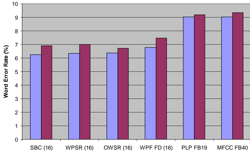
Figure 4. Results for speech frame length of 25.625 milliseconds: The WER for language weight = 9.5 (left bar) and language weight = 12.0 (right bar)
